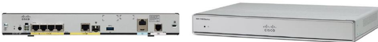
Figure 3. Cisco 1120 and 1160 with LTE pluggable and 802.11ac Wi-Fi options
